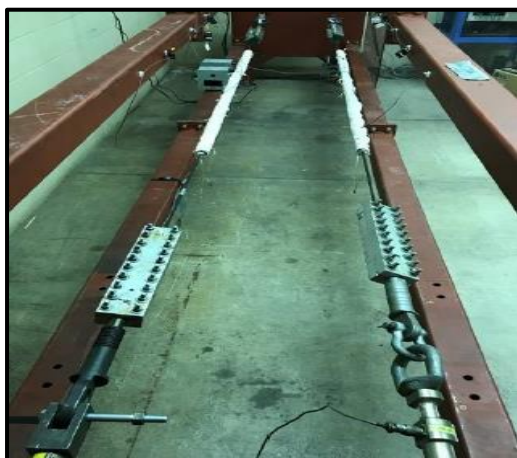
Pic 1: Core installed for heat stress at Kinectrics
